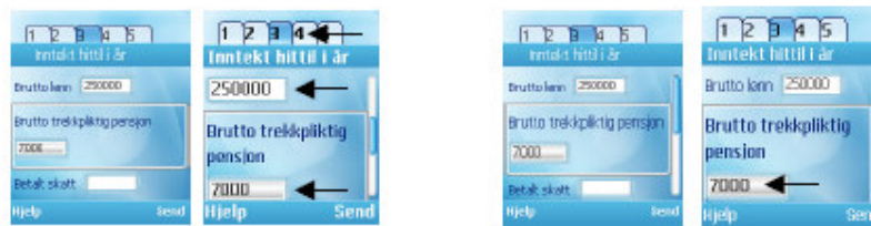
Fig. 5. Changes in the size of the font all over the user interface, or only in selected fields.
